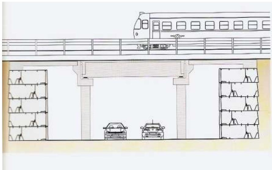
**FOR BRIDGES** Typical Evergreen Maxi Bridge abutment with Pillar and slab support
