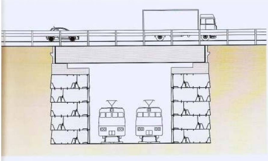
**FOR RAILWAYS** Typical Evergreen Maxi Bridge abutment using gravity walls
