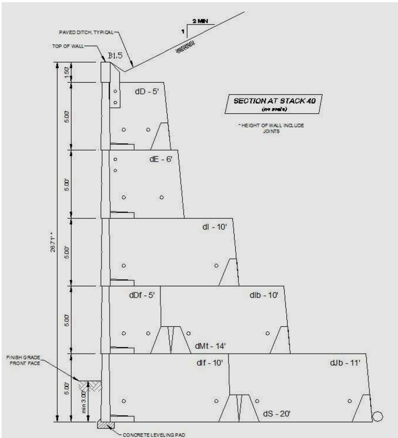
Evergreen Maxi Gravity Retaining wall supporting Railroad surcharges by side by side units in bottom row
